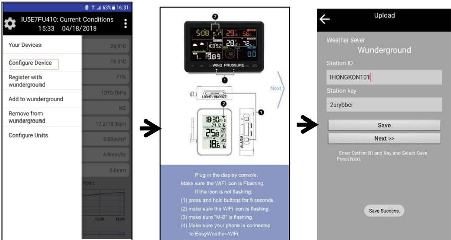
**Figure 13: Mobile application – Provisioning device (Android)**
